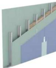
■ Interior partitions constructed with KNAUF W112 dry-wall system, using water-resistant gypsum boards and mineral wool insulation.
