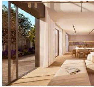
■ Aluminium frames with thermal break technology by Alumil, with double energy-efficient glazing and integrated mosquito screens.
