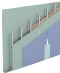
External -internal KNAUF type dry-wall system, including all necessary substructures and finishing works
